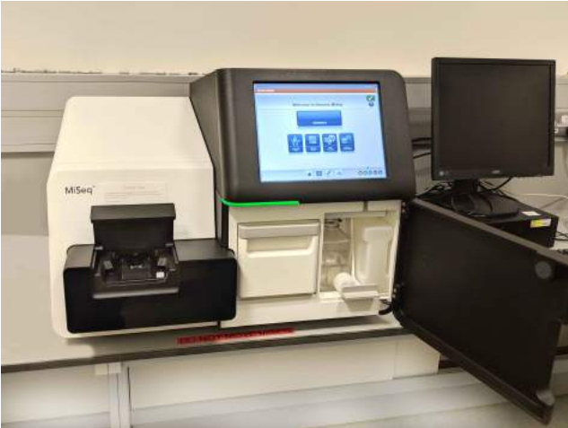
Figure 3: Sequencing platform for the generation of whole genome sequences. Photo: Rosemarie Slowey.
